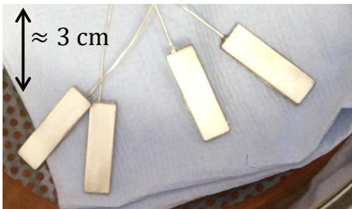
Blocks of sintered silver powder make excellent thermal contact with the refrigerant due to their high porosity and immense service area.
