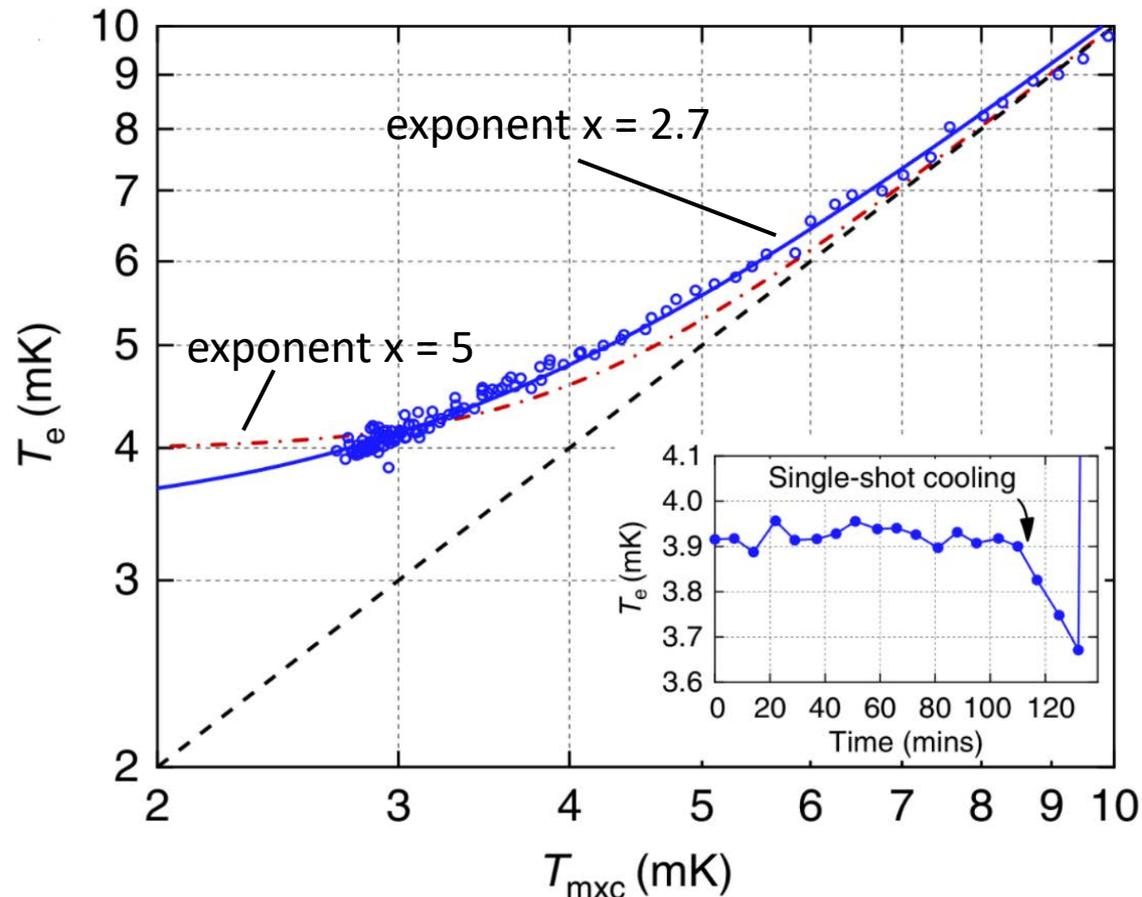
Below 7 mK, the electron temperature reported by the CBT no longer agrees with the temperature of the refrigerator (as measured by a vibrating wire viscometer)
