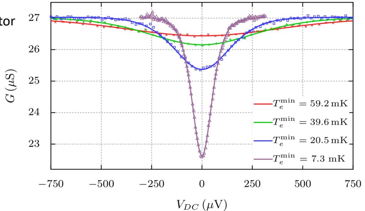
Warmest three isotherms are fitted (simultaneously) to calibrate the CBT. The fit gives  $C_{\Sigma} = 236.6$  fF and  $R_T = 22.42$  k $\Omega$
