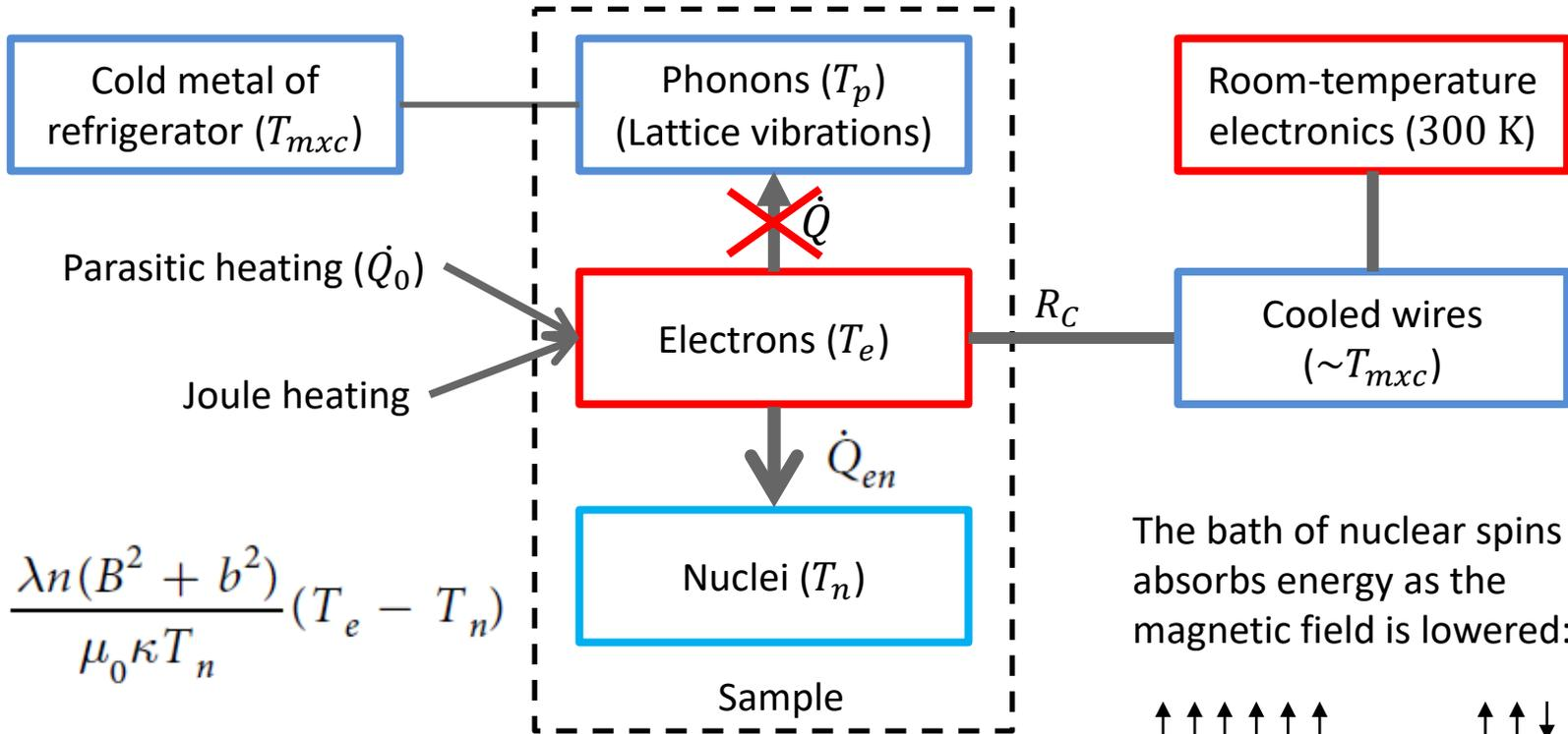
The bath of nuclear spins absorbs energy as the magnetic field is lowered:
