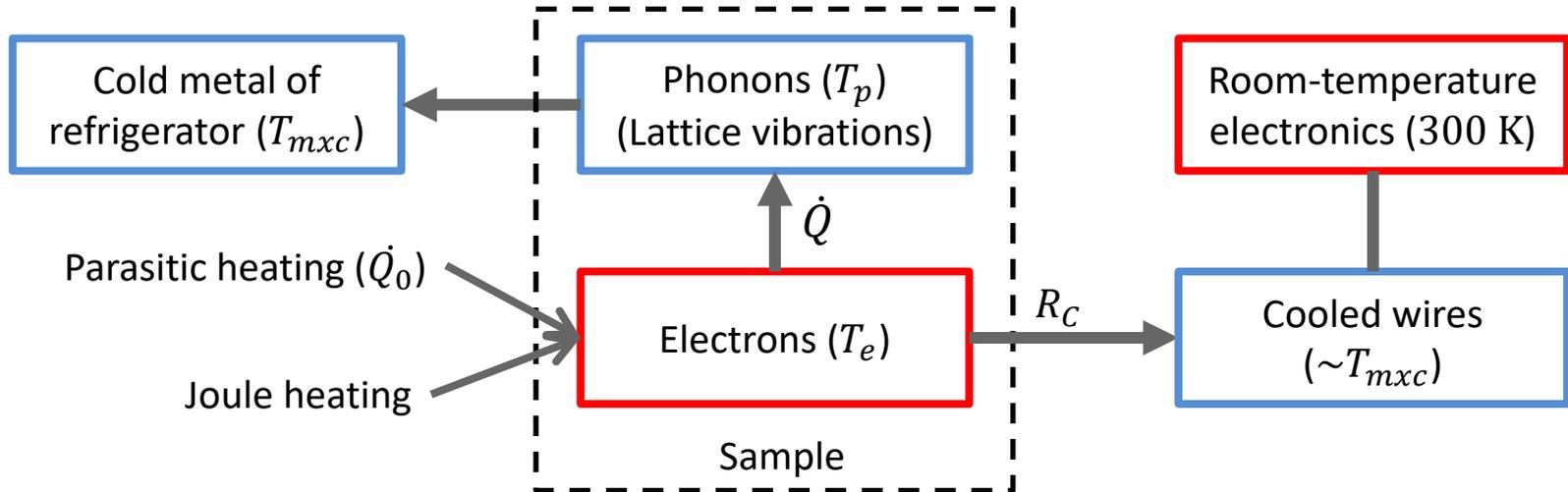
Problem: electron-phonon coupling is very weak in small structures at low temperatures.
