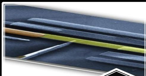
Rectification of electronic heat current by a hybrid thermal diode
