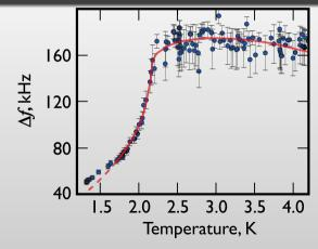
$$\Delta f = C \frac{1}{2} \underbrace{\frac{\rho_n}{\rho_{\text{Al}}} \frac{S}{V} \sqrt{\frac{\eta}{\pi \rho_n f_1}}}_{T} \left(\frac{f}{f_1}\right)^2 f$$
